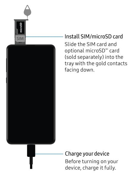
NOTE Use only charging devices and batteries that are approved by Samsung. Samsung charging devices and batteries are designed for your device to maximize battery life. Using other charging devices and batteries may void your warranty and may cause damage.
